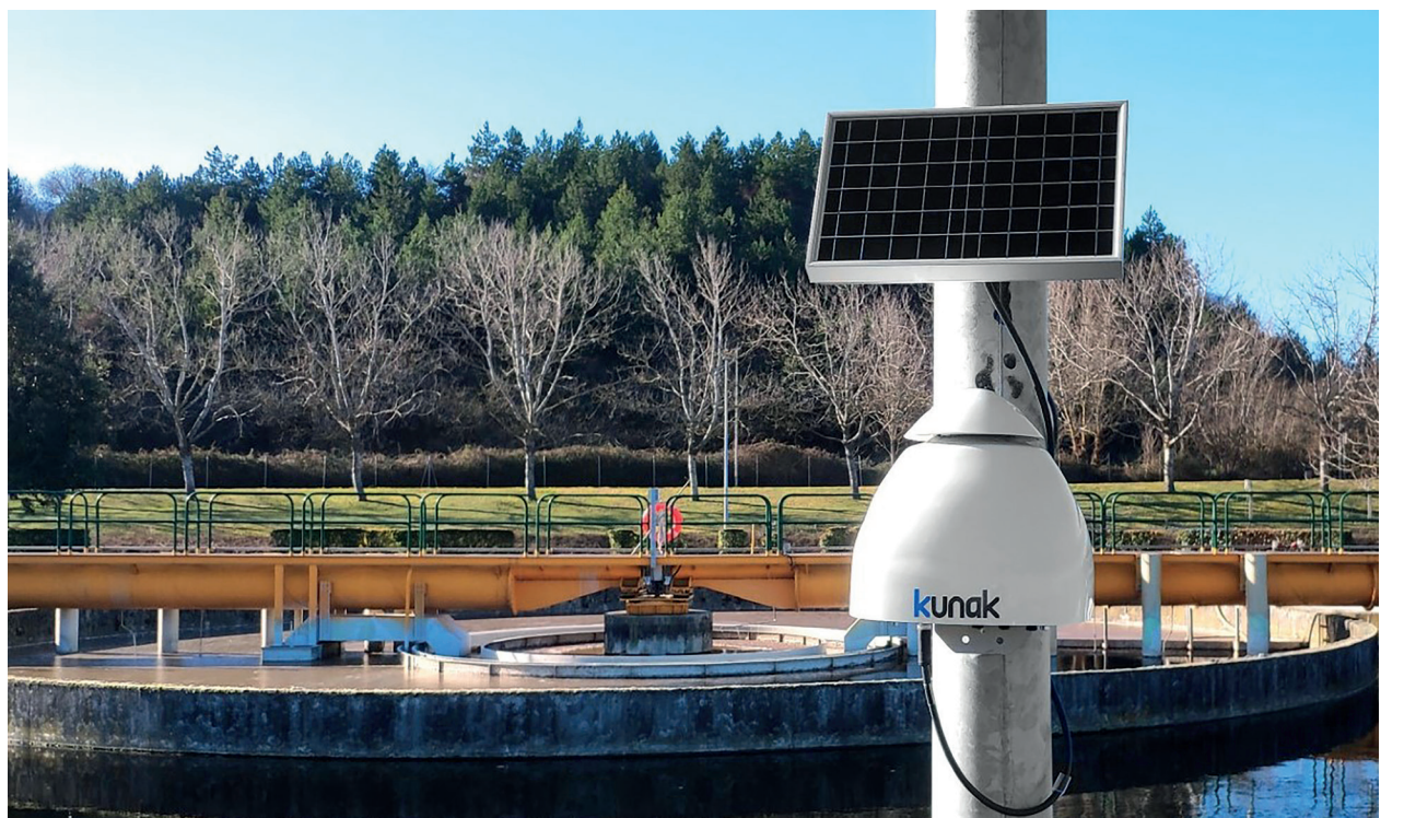
Kunak AIR Pro station in a WWTP
