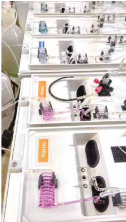
Multiple samples are analysed simultaneously for parameters such as ammonia, nitrate, nitrite, orthophosphate, silicates, total nitrogen and total phosphorus
