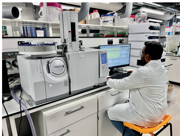
Left: Sachin Solomon (Knowledge Exchange Associate) uses the Shimadzu GCMS-QP2010 SE system with an AOC-20i autoinjector to carry out the GC-MS analysis of pyrolysis bioliqids. Right: Dr Christopher Thomas (Knowledge Exchange Associate) working with EBRI's 'simulated distillation' system, consisting of a Shimadzu Nexis GC-2030 with SimDist software.
