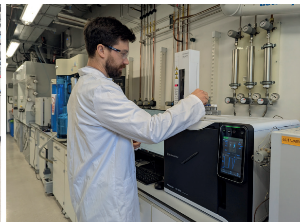
Left: Sachin Solomon (Knowledge Exchange Associate) uses the Shimadzu GCMS-QP2010 SE system with an AOC-20i autoinjector to carry out the GC-MS analysis of pyrolysis bioliqids. Right: Dr Christopher Thomas (Knowledge Exchange Associate) working with EBRI's 'simulated distillation' system, consisting of a Shimadzu Nexis GC-2030 with SimDist software.
