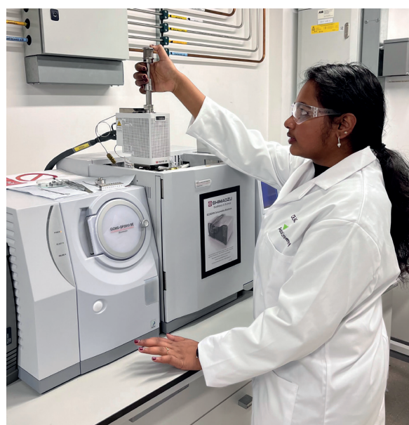
Anitta Xavier (Research Placement Student) injects a biomass sample into a Frontier Lab micropyrolyser for direct transfer to the Shimadzu GCMS-QP2010 SE system.
