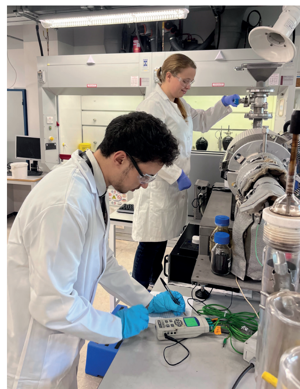
Adam Elaradi (Undergraduate Researcher) and Dr Sarah Asplin (Post-doctoral Research Associate) operate the laboratory-scale intermediate pyrolysis system at EBRI. The system can take up to 300 g/h of biomass, and has a maximum processing temperature of 600 °C.
