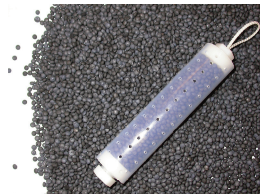
Figure 1. Bio-Traps ® samplers available from EnviroGene Ltd, allow the collection of active microorganisms that form biofilms on submerged surfaces.
