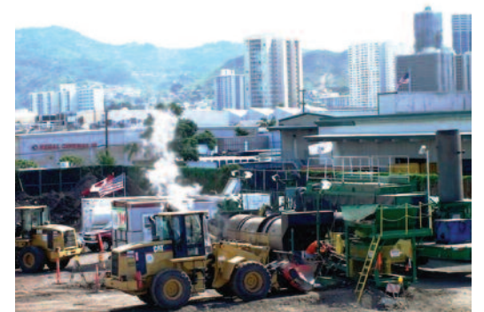
Fig 2. Loading contaminated soil into MTSR system, Honolulu, Hawaii
