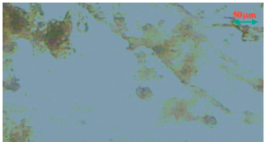
Figure 2: Thickened mixed sludge, with thermal hydrolysis at 165°C in 20 minutes – without pressure drop
