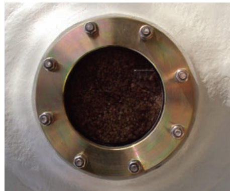
Figure 6: Lentikats Biocatalyst inside a reactor.
