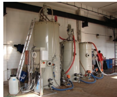
Figure 5: A pilot-scale test unit (nitrification – denitrification – retention).
